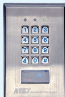
DK-2882A/B MK-II+ (Three Outputs, Wiegand, IP-66)
