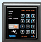
DK-2872 MK-II+ (Three Outputs, Wiegand, IP-55)
